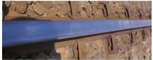
Fig. 10: Status of the Generation of Undulatory Wear
