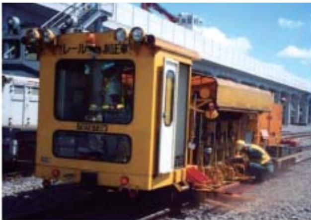
Fig. 12: Rail Grinding Car of a Domestic Manufacturer
