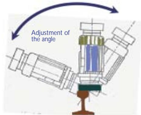
Fig. 13: Angle between a Rail and the Abrasive Grindstone
