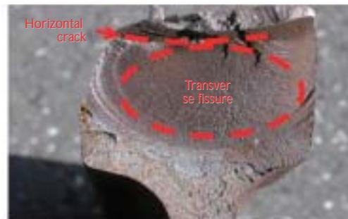
Fig. 6: Crack that has Progressed to the Interior of the Rail
