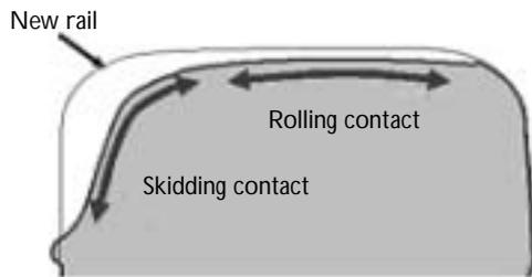
Fig. 7: State of Contact of the Outer Rail
