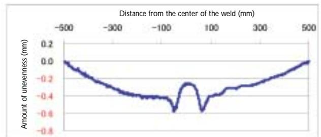
Fig. 4: Unevenness of the Welded Part of a Rail
