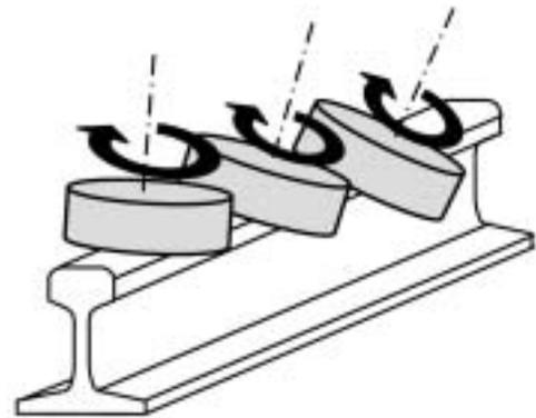
Fig. 14: Deployment of the Abrasive Grindstones on a Rail Grinding Car
