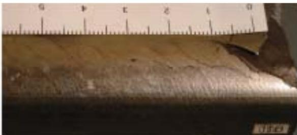
Fig. 9: External Appearance of a Head Check
