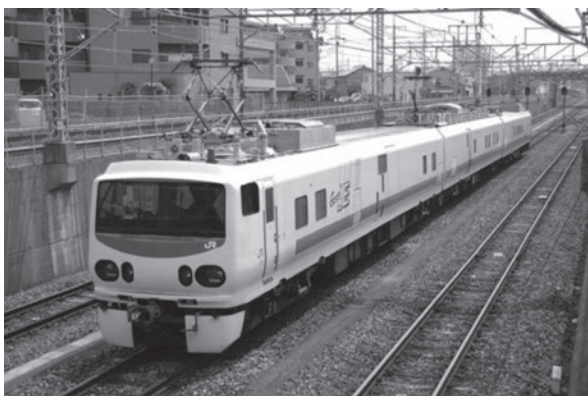
Fig. 1 Electric and Track Inspection Car for Conventional Lines (East-i)
