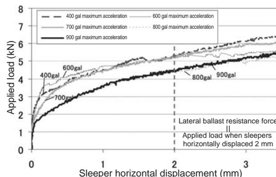
Fig. 8 Results of Lateral Ballast Resistance Force Measurement (Example at 1 Hz Frequency)
