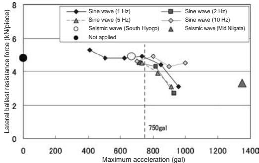
Fig. 9 Lateral Ballast Resistance Force per Frequency
