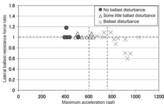
Fig. 10 Lateral Ballast Resistance Force Ratio and Maximum Acceleration
