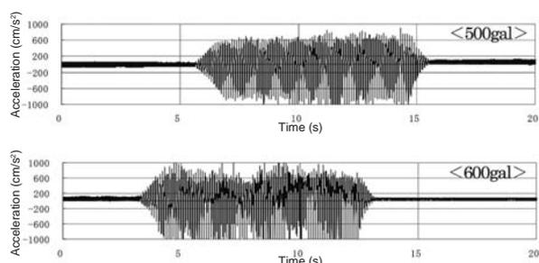
Fig. 6 Acceleration at Ballast Slope (10 Hz, 500 gal & 600 gal)
