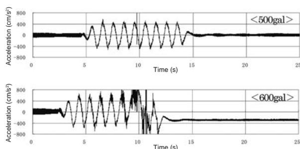
Fig. 5 Acceleration at Ballast Slope (1 Hz, 500 gal & 600 gal)
