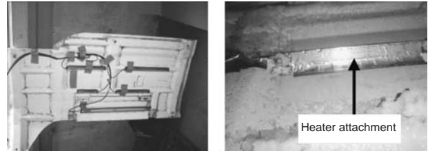
Fig. 3 Bogie Cover Snow Melting Heater
