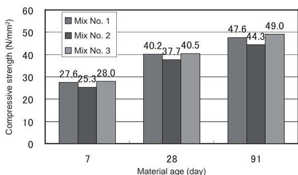
Fig. 4 Compressive Strength Test Results
