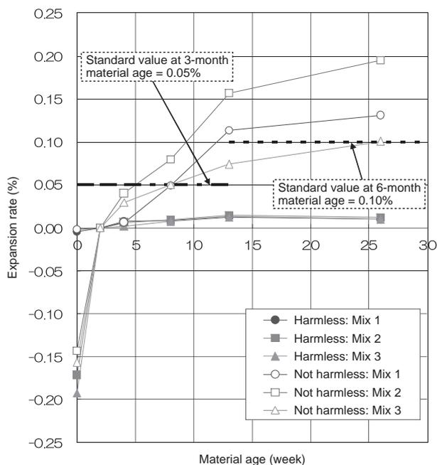
Fig. 7 Mortar-Bar Method Test Result
