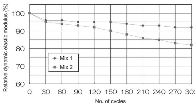
Fig. 5 Freezing-Thawing Test Results (Relative Dynamic Elastic Modulus)
