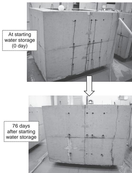
Fig. 11 Change of Leakage from Square Tank Test Sample (Mix 2)
