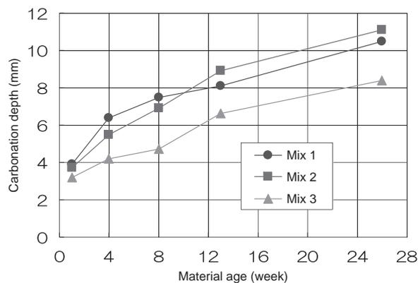
Fig. 6 Accelerated Carbonation Test Results
