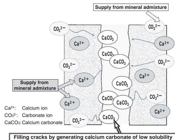
Fig. 2 Mechanism of Self-healing Concrete
