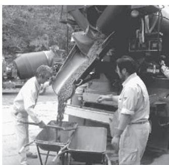
Fig. 10 Discharging from the Agitator Truck (Test Concrete)
