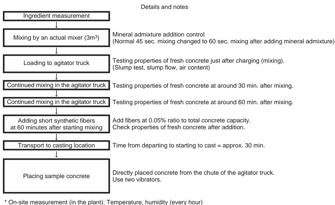
Fig. 9 Test Flow of Actual Mixer-Mixed Self-Healing Concrete
