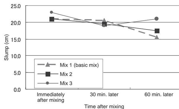
Fig. 8 Slump Change Over Time
