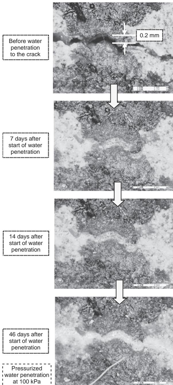
Fig. 3 Example of Crack Filling (With Mix Proportion Shown in Table 1)
