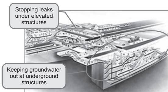
Fig. 1 Application of Self-Healing Concrete to Railway Structure
