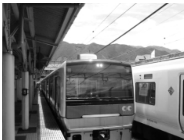
Fig. 4 Communications test utilizing a satellite (rooftop of car No. 1)
