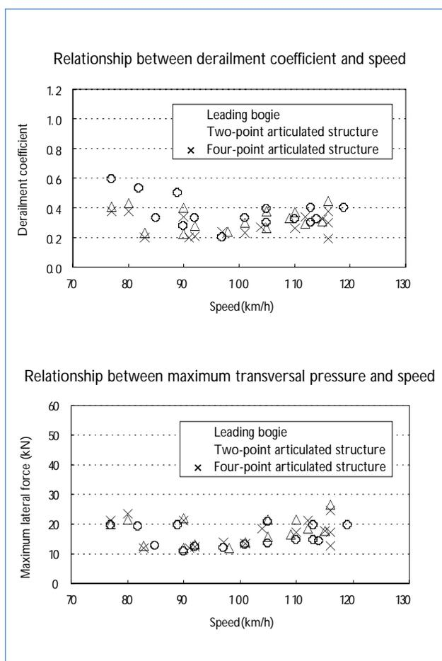
Fig. 13 Derailment coefficient and maximum lateral force ( $R = 800$  m and  $C = 95$  mm)
