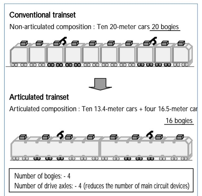
Fig. 1 Reduced number of bogies in articulated structure
