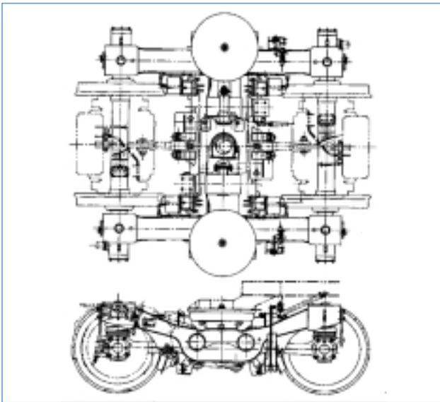
Fig. 3 Two-point support articulated bogie
