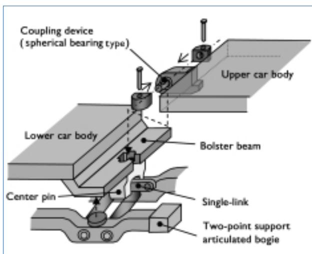
Fig. 5 Mounting the two-point support articulated bogie
