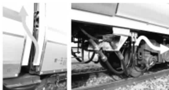
Fig. 12 End-to-end cable routing (left) and bogie-internal cable routing (right)
