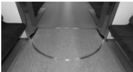
Fig. 11 Semicircular apron mechanism
