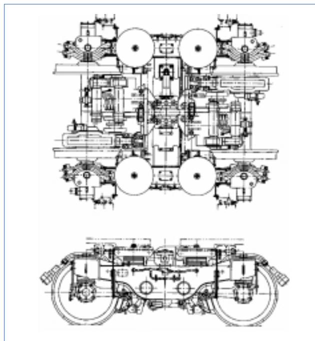
Fig. 6 Four-point support articulated bogie
