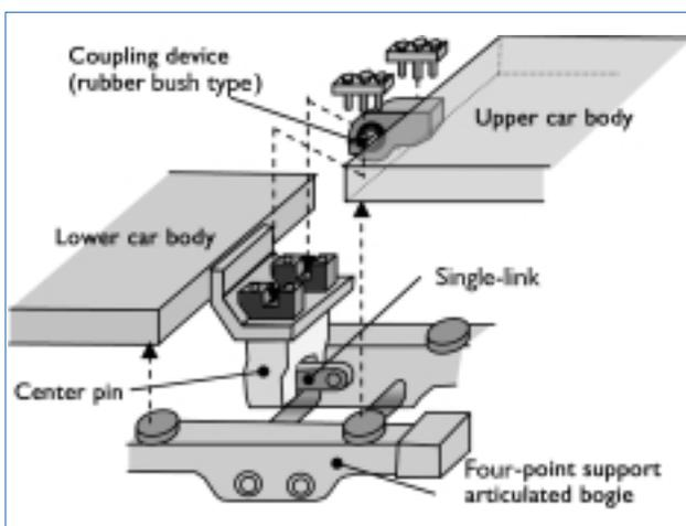
Fig. 7 Installation of four-point support articulated bogie
