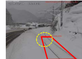
図-4 支障物捕捉例[左:落雪(昼)]
