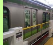
“Smart” automatic platform gates
