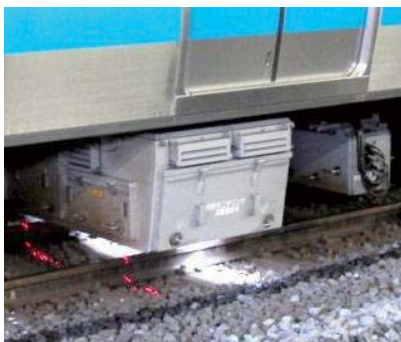
Train track facility monitoring equipment
