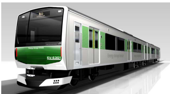
Catenary and battery-powered hybrid railcar system on the Karasuyama Line
