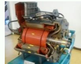
Cut model of railcar electric motor
