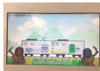
Series EV-E801 railcar's energy flow monitor
