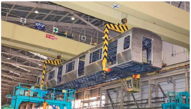
Assembling a railcar body structure
