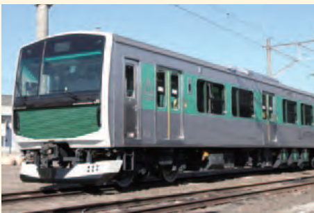
ACCUM catenary and battery-powered hybrid railcar
