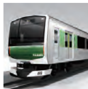
Catenary and battery-powered hybrid railcar train
