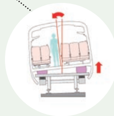
Car body tilting system
