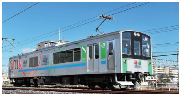
A catenary and battery-powered hybrid railcar
