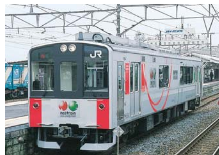
Hybrid railcars that employ fuel cells
