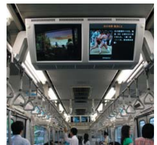
Ceiling-mounted digital video monitors on a Keihin-Tohoku Line train
