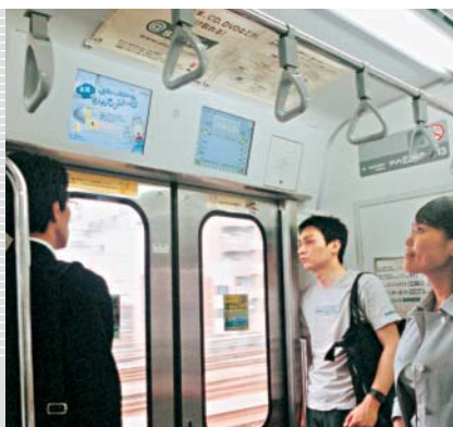
E231 series railcar's 15-inch visual displays on the Yamanote line
