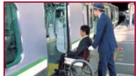
Entry/exit steps for passengers in wheelchairs The AC Train, a next-generation commuter train system, has specially designed steps to facilitate wheelchair accessibility.
