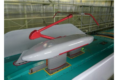
E5 Series trains have low-noise pantographs
