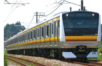
E233 series: VVVF inverter cars for commuter and suburban transportation
