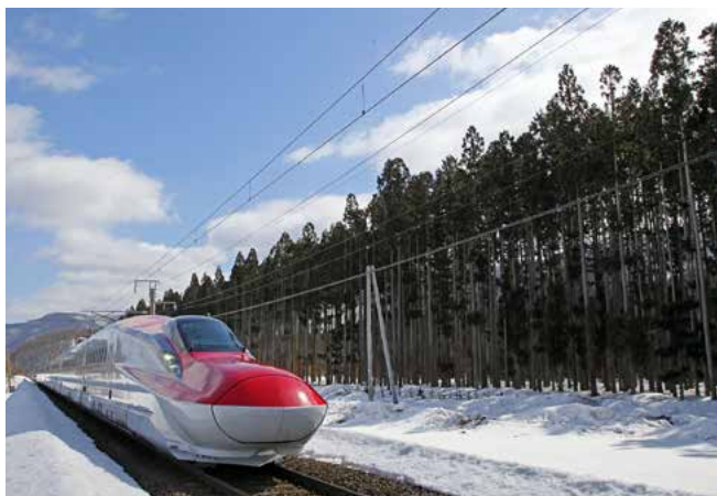
Sashimaki No.1 railway forest on the Tazawako Line (forest to protect against blizzards)
