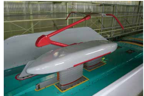
E5 Series trains have low-noise pantographs
