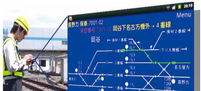
Visualization of maintenance work procedures
