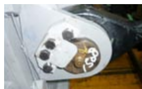
Metal fittings to prevent unfastening of the pins that support reduction gears
