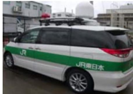
An automobile with on-board satellite communication facilities
