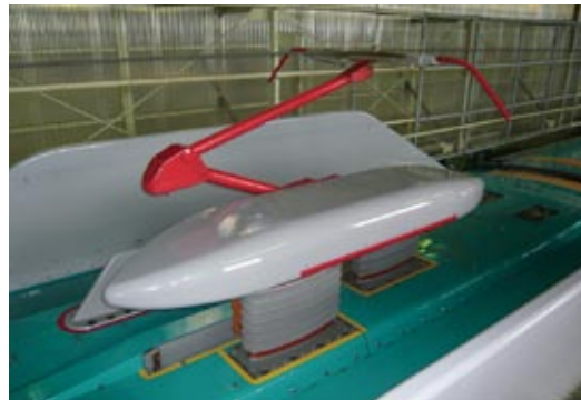
E5 Series trains have low-noise pantographs
