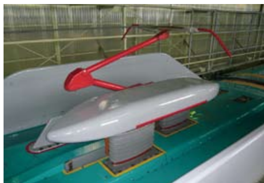
E5 Series trains have low-noise pantographs
