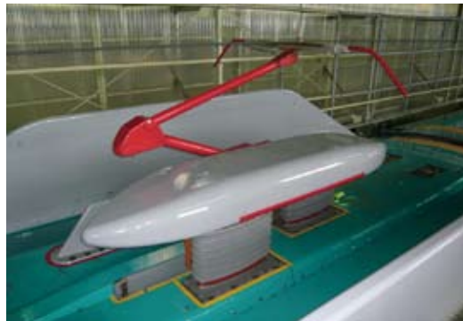
E5 Series trains have low-noise pantographs
