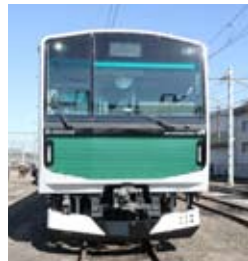
EV-E301 Accumulator System (ACCUM) train
