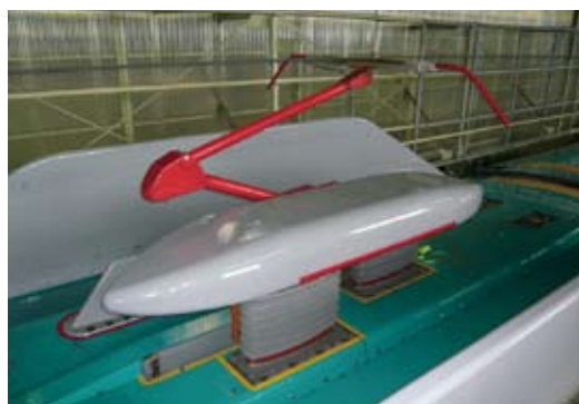
The E5 Series employs low-noise pantographs
