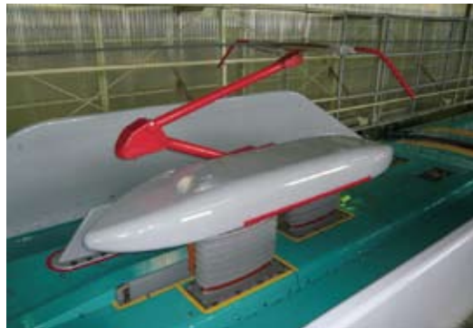
The E5 Series employs low-noise pantographs.
