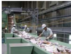
Bldg. B - Manual segregation of newspapers and magazines line
