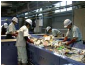
Bldg. A - Manual segregation of mixed trash line
