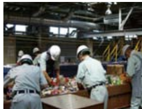
Bldg. A - Manual segregation of cans and bottles line
