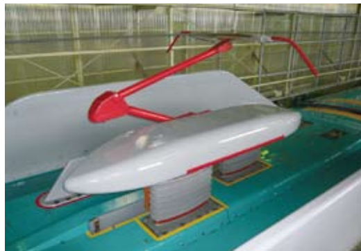
The E5 Series employs low-noise pantographs.
