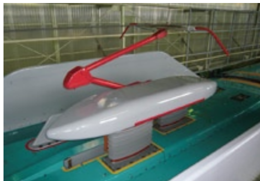
The E5 Series employs low-noise pantographs.
