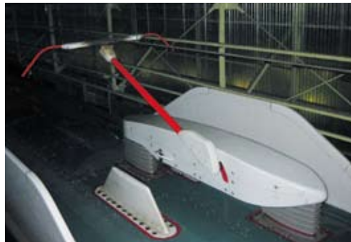
Test train "FASTECH" uses a low-noise single arm pantograph.
