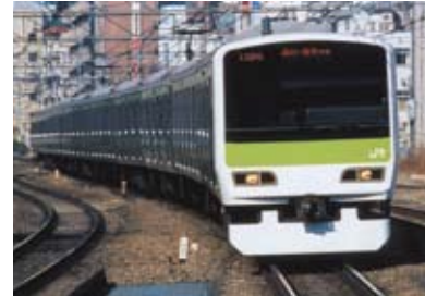
E231 series: VVVF inverter cars for commuter and suburban transportation.
