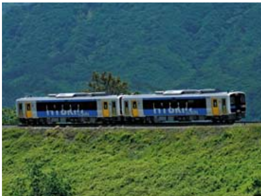
The world’s first diesel hybrid railcars operating on the Koumi Line
