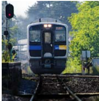
The world's first diesel hybrid railcars operating on the Koumi Line
