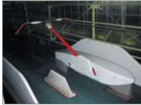
Test train "FASTECH" uses a low-noise single arm pantograph.
