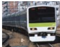
E231 series: VVVF inverter cars for commuter and suburban transportation.
