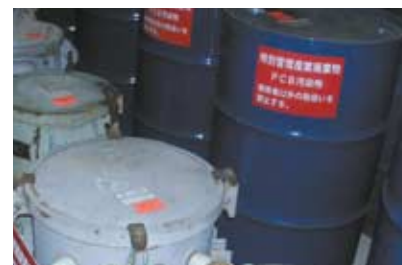
PCBs are kept in special storage under stringent control
