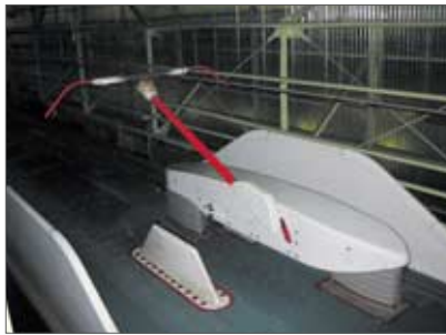
Test train "FASTECH 360" uses a low-noise single-arm pantograph.
