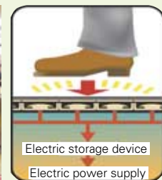
Mechanism of the power-generating floor
