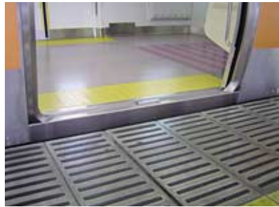
Car doors with reduced difference from platform levels
