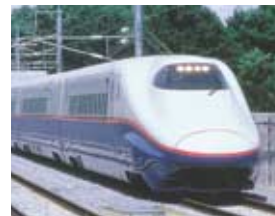
E2 series: VVVF inverter railcars used for Shinkansen "Asama" and "Hayate" trains.
