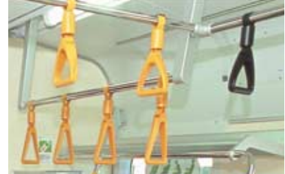
Lower overhead luggage racks and supports for standing passengers in priority seat areas and in women-only cars
