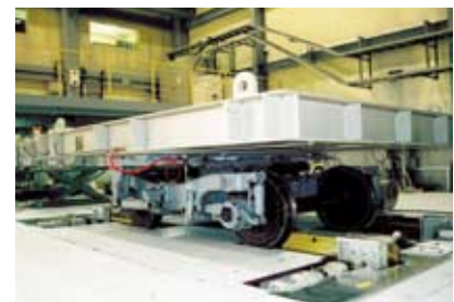
Test facility in the Research & Development Center of JR East Group (bogie testing equipment)
