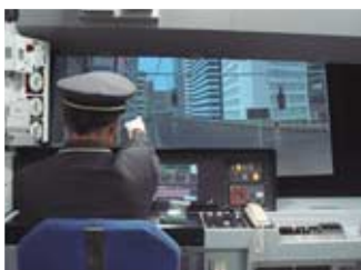
“Train operation simulator”: accident prevention by training with a feeling of driving a real train
