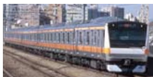
The E233 Series, with duplication of major equipment to increase resistance to failures
