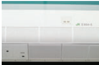
Sound absorbent plates are installed on the bottom and lower side of prototype high-speed Shinkansen FASTECH 360 to reduce noise.
