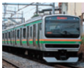
E231 series: VVVF railcars that are mainly used as commuter or suburban trains.
