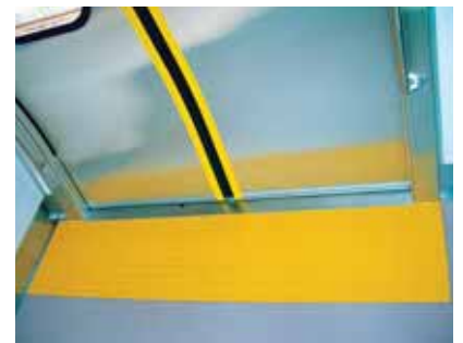
Features on the new E531-series railcars on the Joban Line include high-visibility coloring around doors, and toilets compatible with electric wheelchairs.
