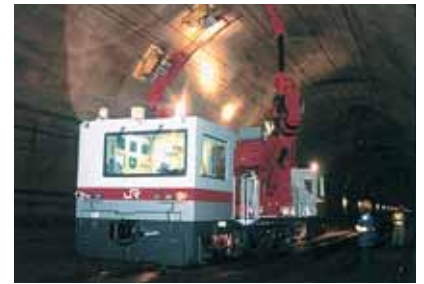
The Tunnel Wall Inspection Vehicle inspects Shinkansen tunnels with precision and efficiency.
