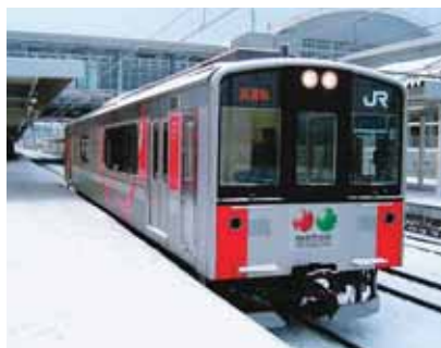
The NE Train, equipped with improved storage batteries for even better performance, being tested in winter conditions.
