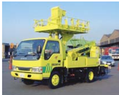
A low-noise rail track vehicle for overhead wire work operates using batteries with a high degree of quietness
