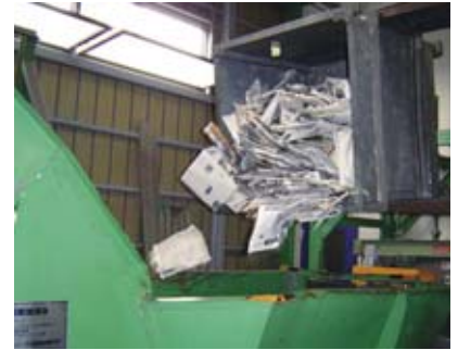
The Shinkiba Recycling Center sorts and compresses discarded newspapers and magazines to be recycled as copy paper
