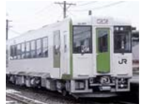
Kiha 110 series: diesel railcars for conventional lines feature fuel-efficient and low-polluting engines
